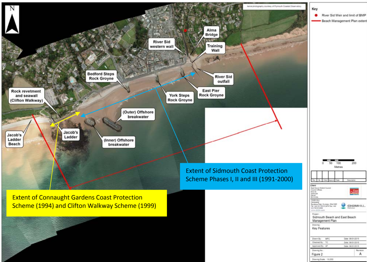
Figure 2-1 Key features and approximate scheme extents along the Sidmouth & East Beach Management Plan extent
