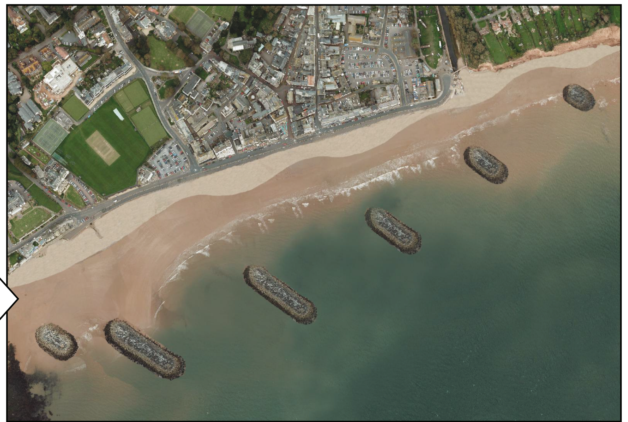
Illustration of how replacing the groynes with additional shore-parallel offshore breakwaters could look (basis of core appraisal)
