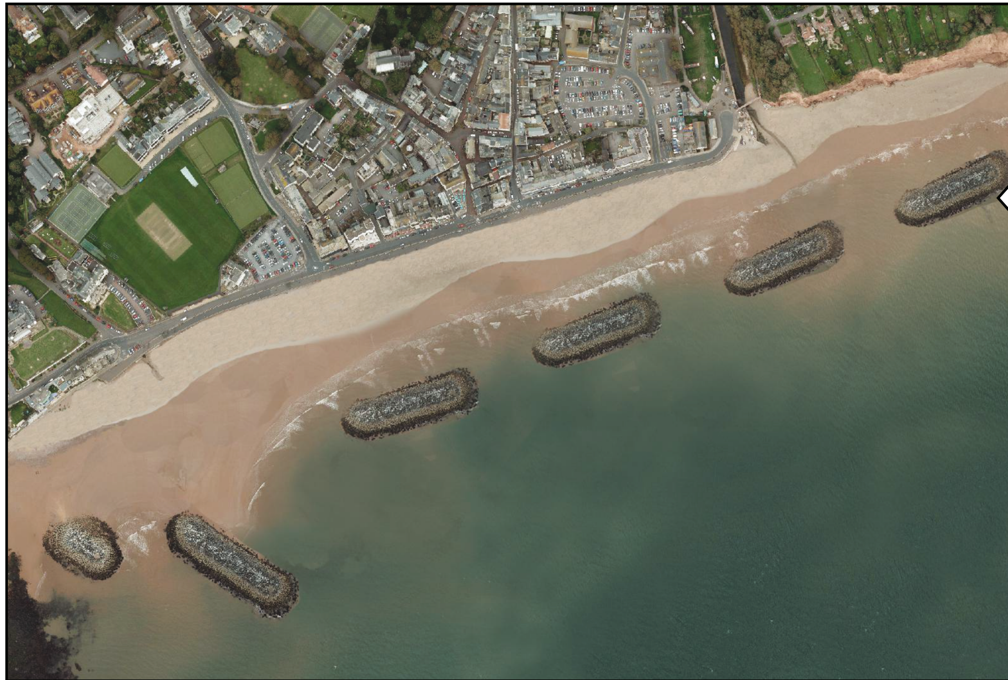
Illustration of how replacing the groynes with additional oblique offshore breakwaters could look (basis of sensitivity test)
