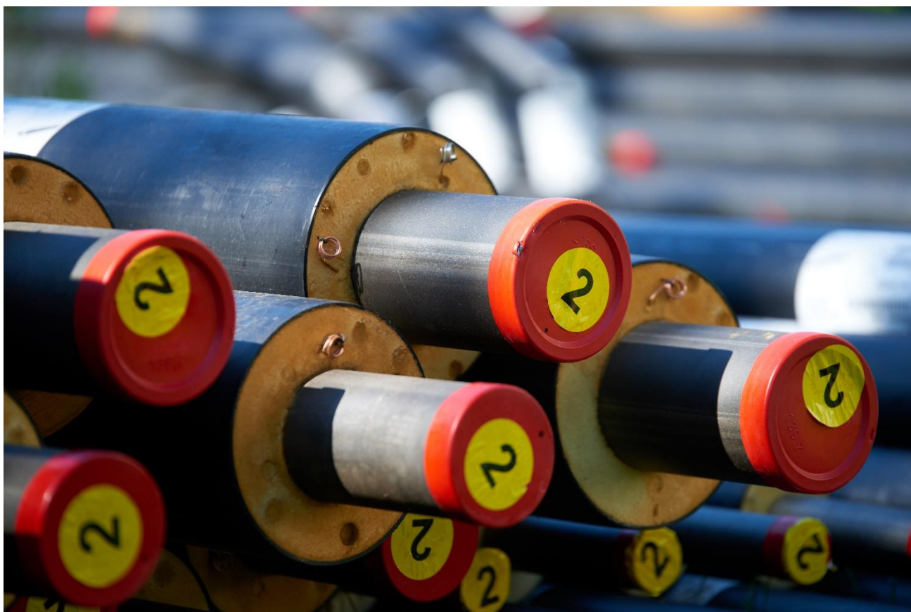
District heating network pipes waiting to be installed
