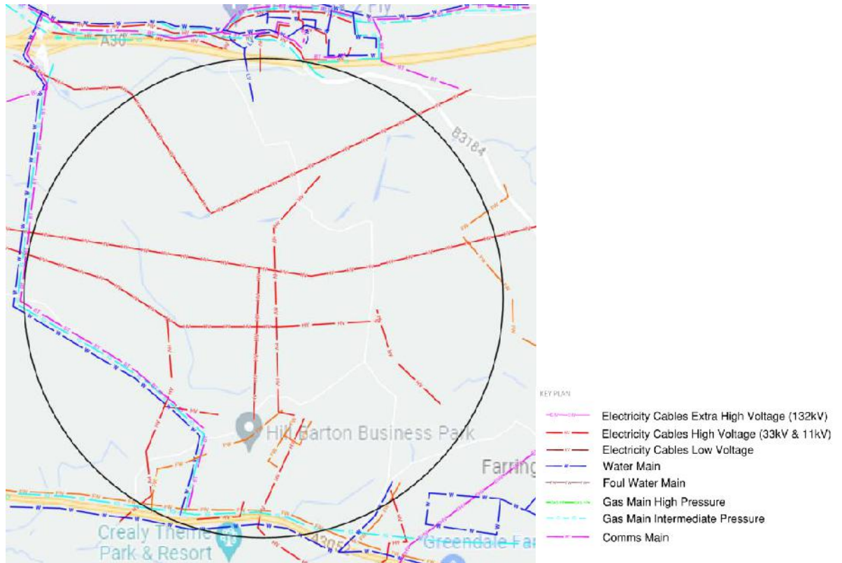
Figure 9.2 – Option 1 Existing Utility Infrastructure
