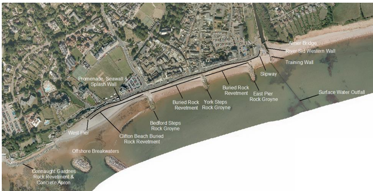
Figure 2.1 Sidmouth's current coastal defence arrangements
