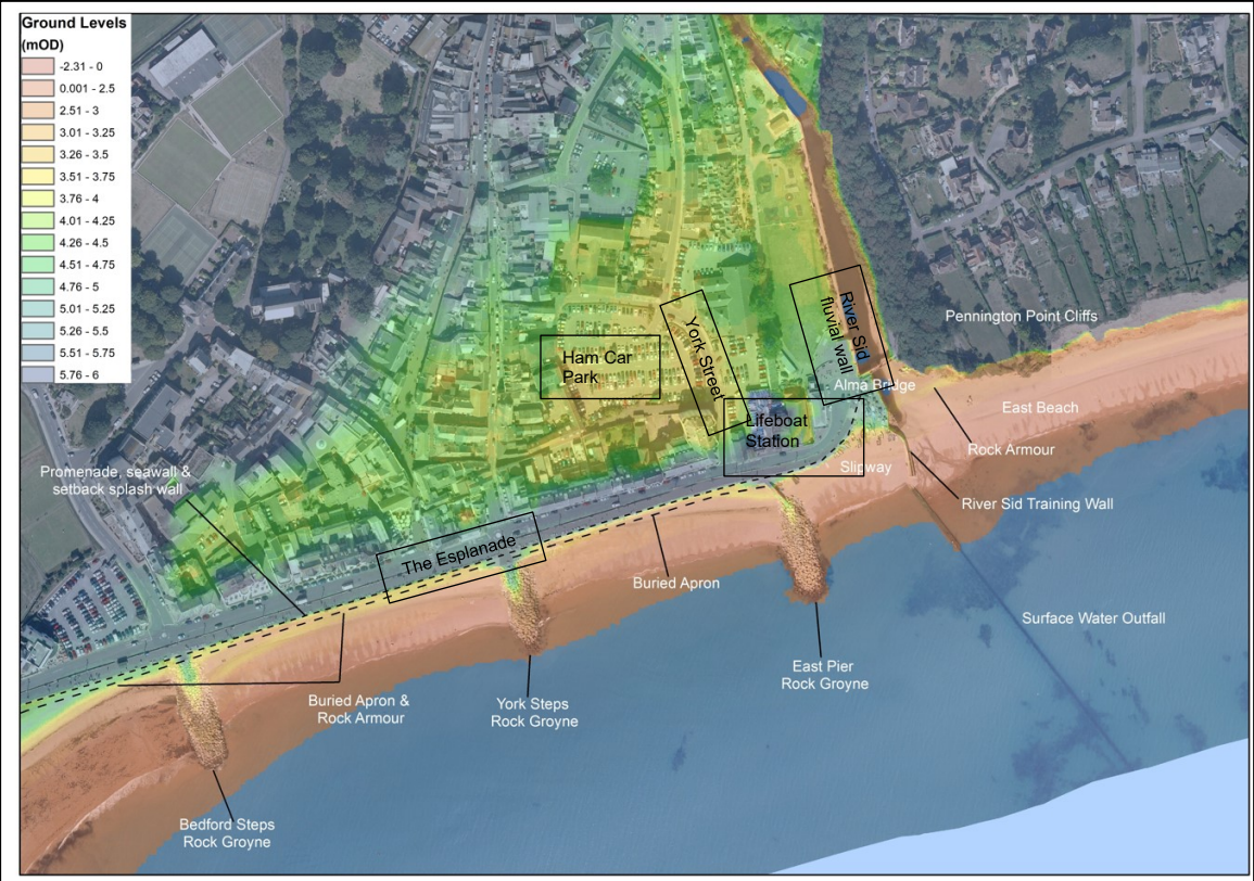
Figure 2: Sidmouth’s existing coastal defence arrangement
