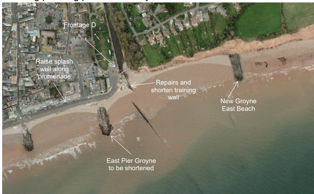
Figure 25: Option S1 showing one new groyne on East Beach
