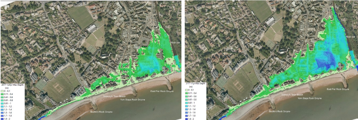
Figure 20: 2017 (left) and 2117 (right) 5% AEP flood extent and depth
