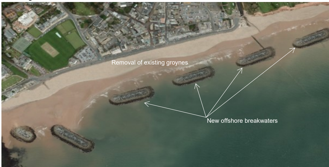
Figure 28: Option S4 comprising four new offshore breakwaters
