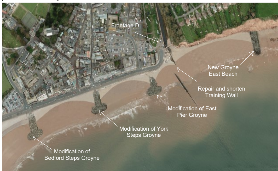
Figure 26: Option S2 showing T-head groynes and additional groyne on East Beach
