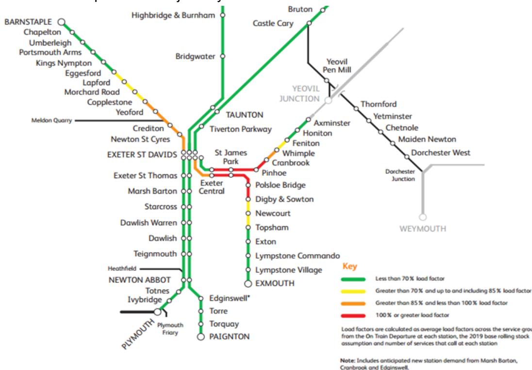
Figure 8.5: Estimated 2023 Load Factor from the 2015 Western Route Study on services arriving into Exeter St David's in AM peak
