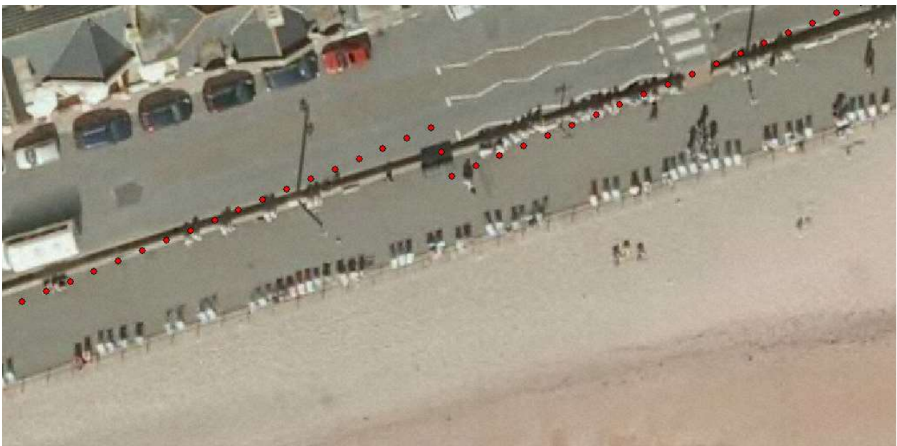
Figure 3-19: Defence Z-Lines within the TuFLOW model
