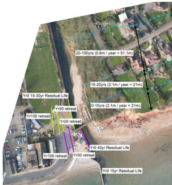
Figure 3-20: Do Nothing cliff retreat and defence failure over 100 years.
