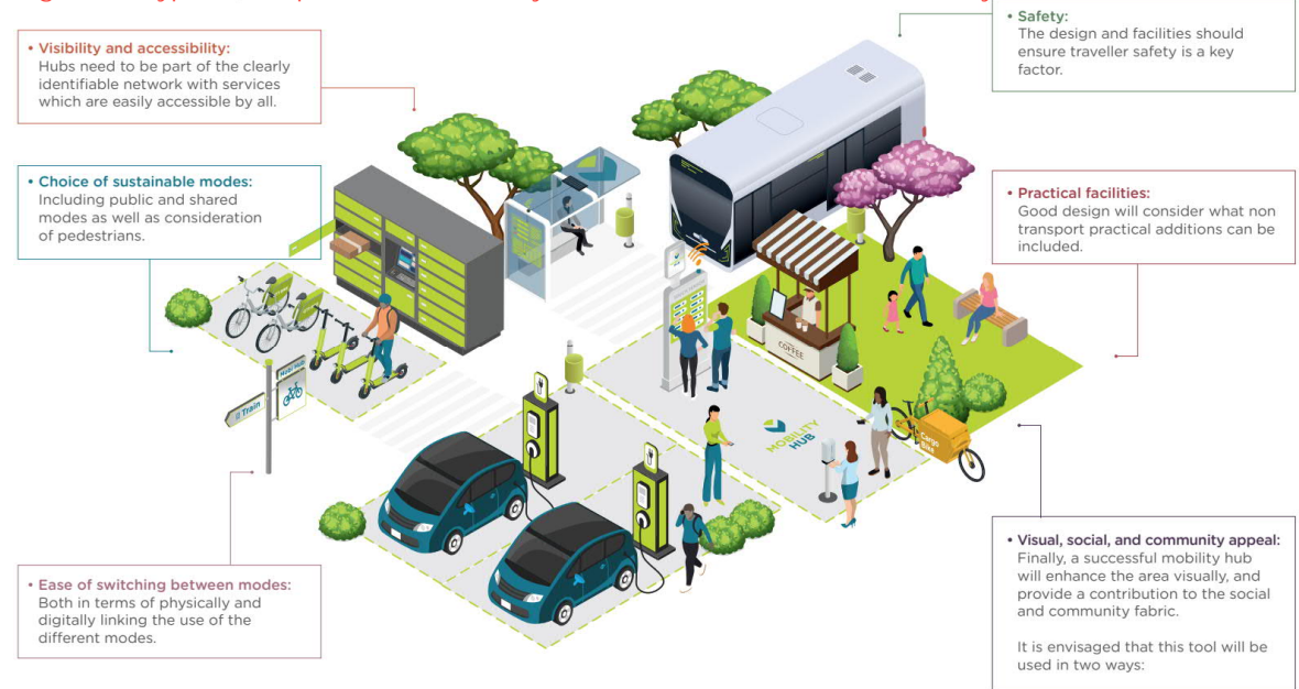
Figure 4.1 Typical components of mobility hubs. Source: CoMoUK UK Mobility Hub Guidance
